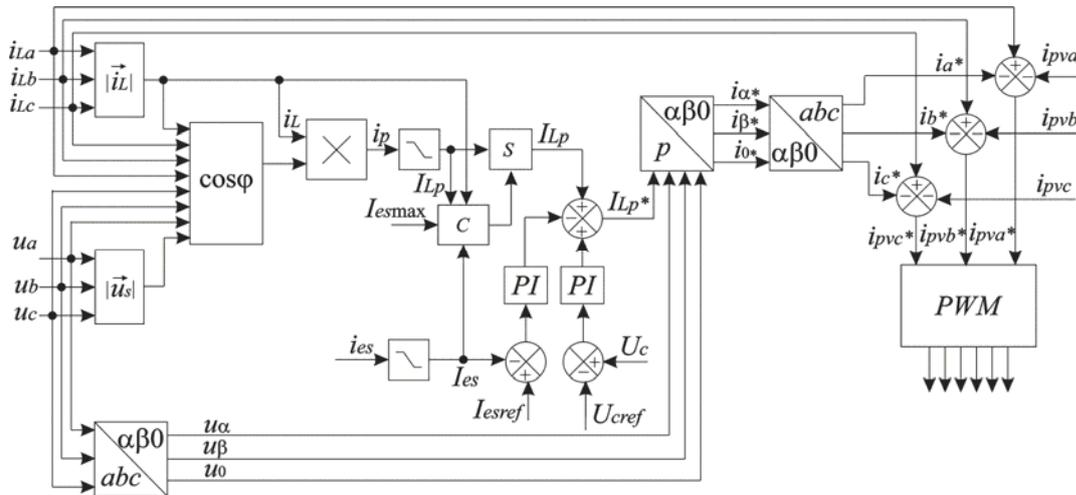
Figure 2. Structural diagram of the control system
