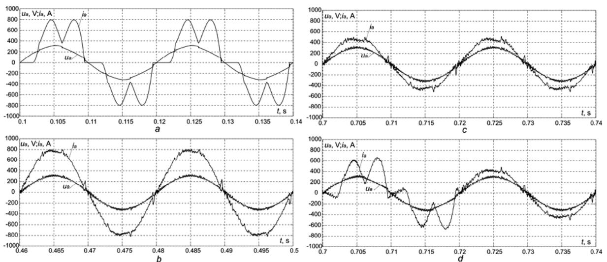
Figure 4. Oscillograms of network voltage and current in phase A
