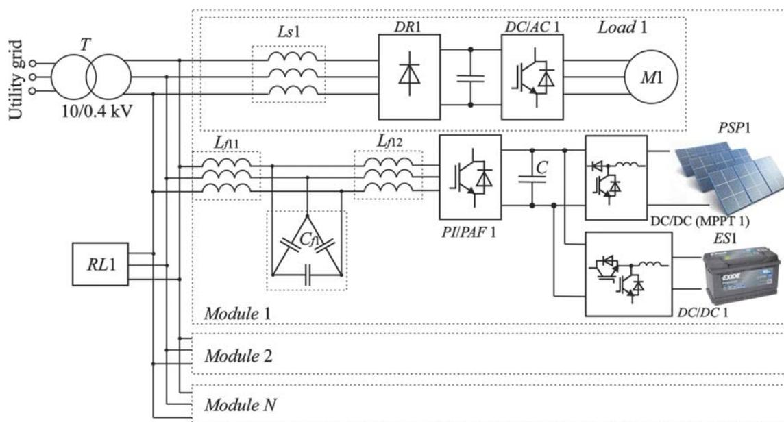
Figure 1. The block-diagram of the power supply system
