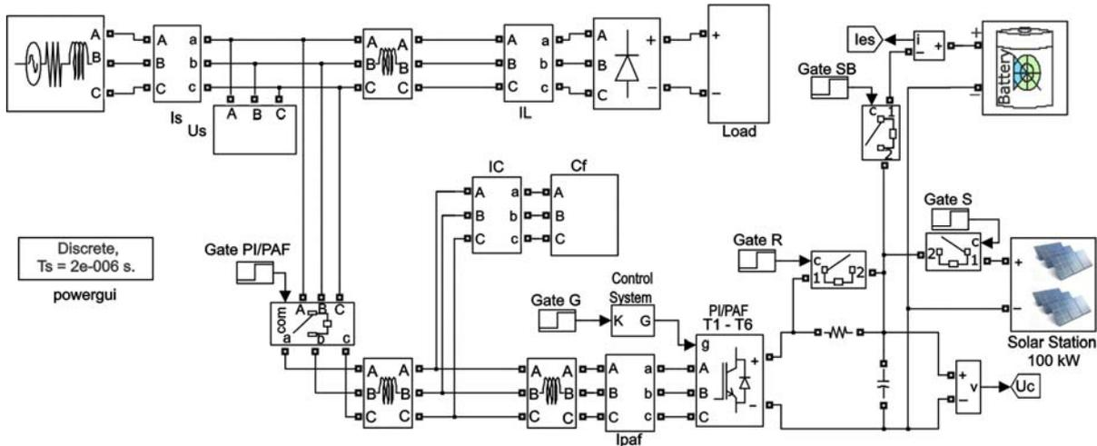
Figure 3. Matlab- model of the distributed power supply system with a solar power plant
